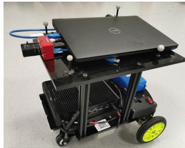
**Figure 5.** AGV equipped with a forward-facing event camera for vehicle motion estimation.
